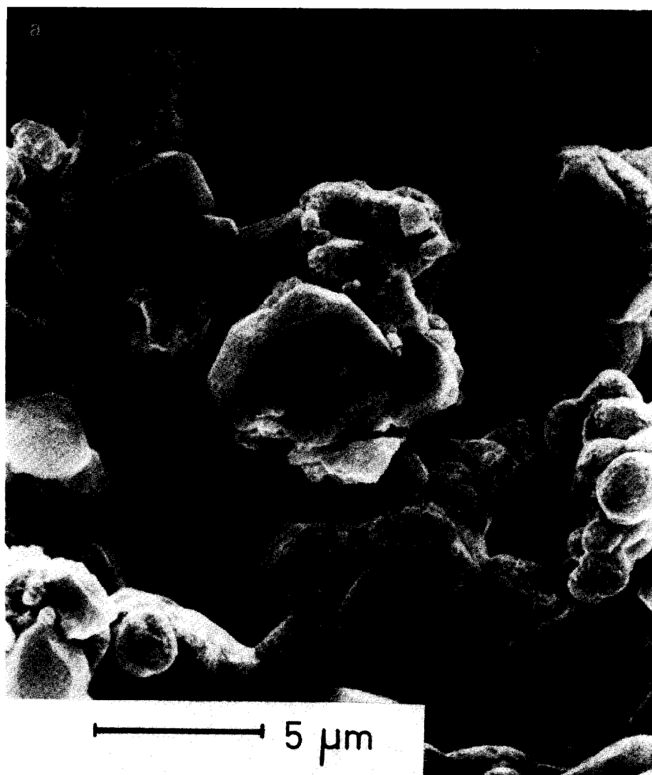
FIG. 5. Scanning electron micrographs of Ag-Sch-9 catalyst after epoxidation at 543 K for 2 days.
