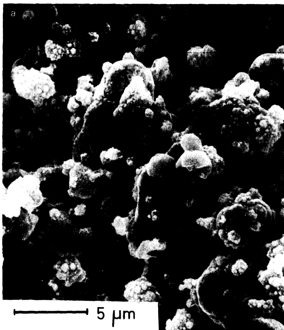
FIG. 4. Scanning electron micrographs of fresh Ag-Sch-9 catalyst.
